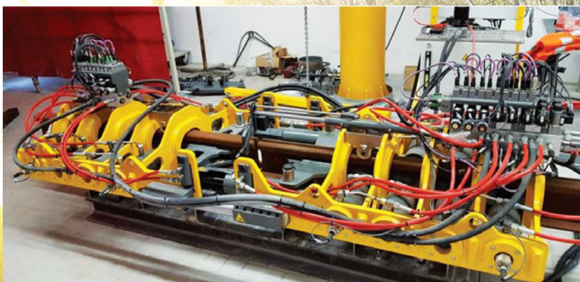
Based on its uses <Aligning, Forging and Shearing> this equipment has been nicknamed ALFONS
