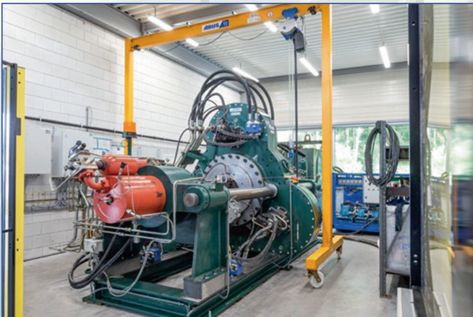
Large industrial prototype machine for orbital friction welding of rails
