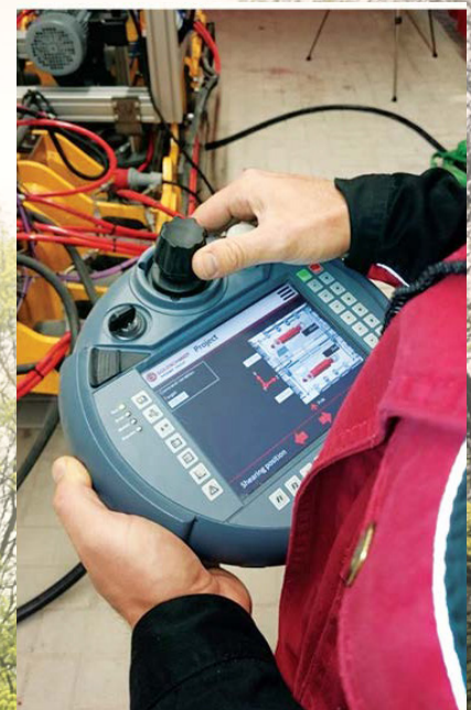
The second development is a process and machine control system that collates all the incoming data from the welding process and generates and documents the manual inputs of the operator, the specified process parameters and the measured values from sensors during the sequence of the automated process steps.
