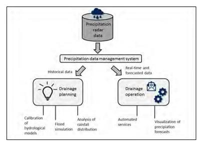
Figure 18: Vision of future drainage management in the Wesermarsch using precipitation radar data.
