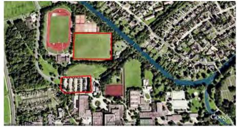
Figure 16: Sports field as flood control area in the proximity of the drainage canal.
