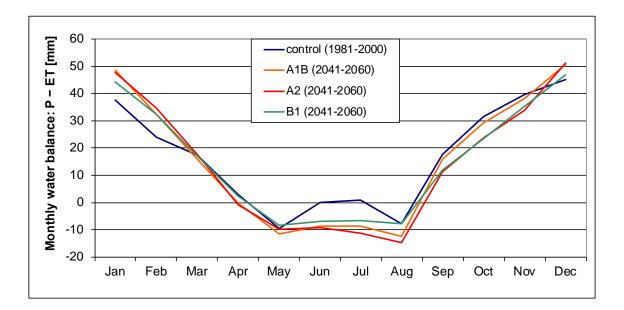
*Figure 9: Water balance projections (precipitation–evapotranspiration) of a physically based hydrological model based on WETTREG climate projections for the Wesermarsch (IPCC scenarios A1B, A2, B1). Source: Bormann et al. (2012).*
