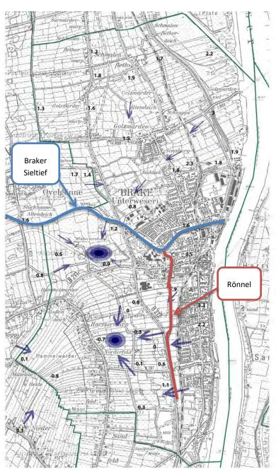
*Figure 7: Topography of the City of Brake; arrows showing the normal flow direction of the surface water.*
