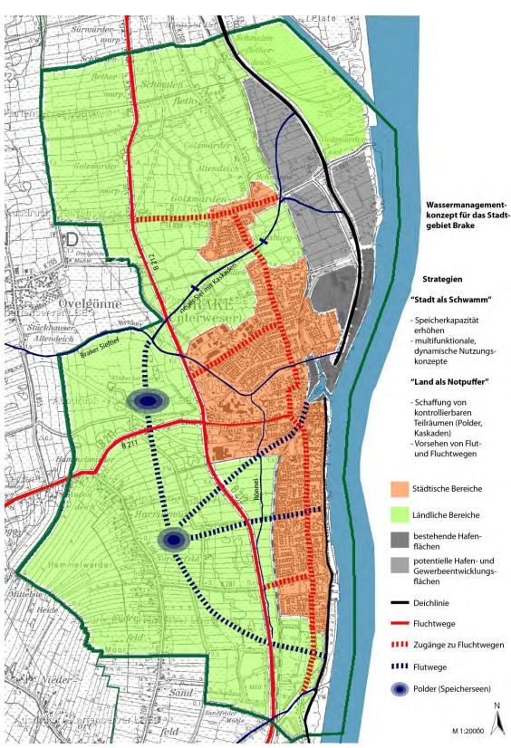
Figure 17: Draft of the urban drainage solution options within the EU Interreg IVB project CPA (in German).
