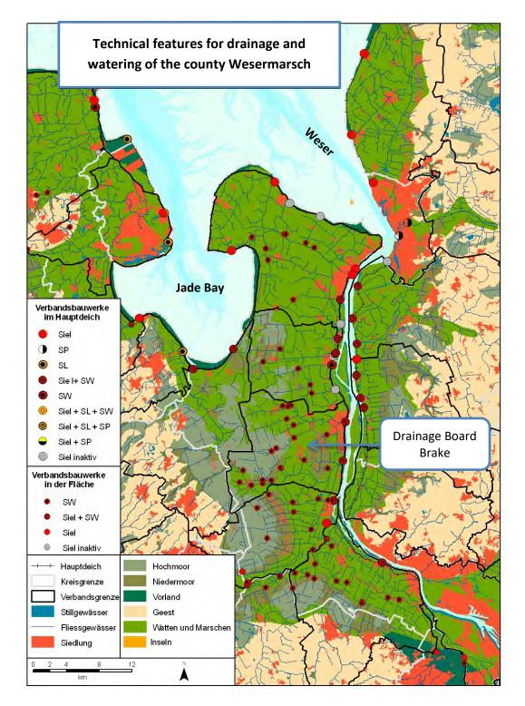
Figure 6: This map shows the water boards and the technical features to ensure the drainage and watering of the northern part of the county Wesermarsch. Source: modified after Ahlhorn et al. (2010)
