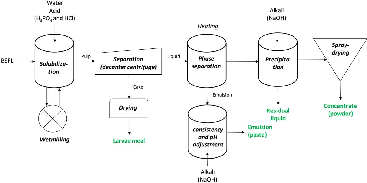
**Figure 18: Process flow chart – pilot processing of BSFL**
