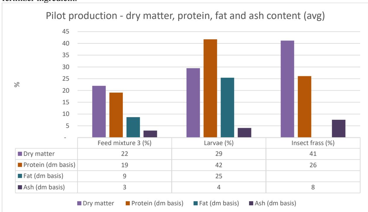
**Figure 15: Content of dry matter, protein, fat and ash in the feed mixture, larvae and insect frass from the pilot production.**
