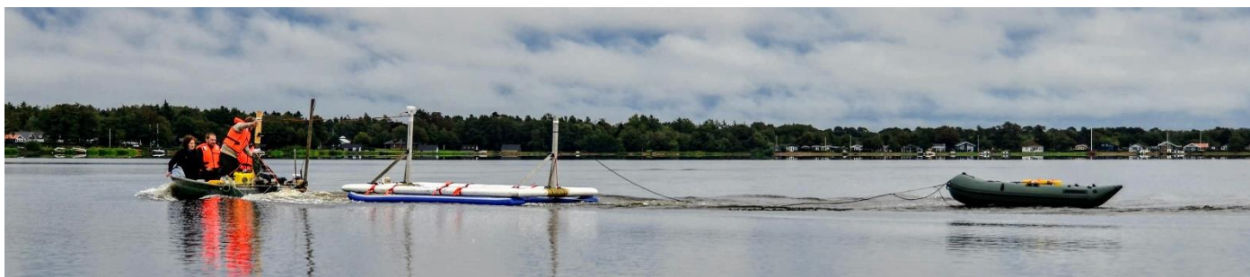
Figure 2. The FloaTEM system. The transmitter coil is mounted on two SUP-boards and the receiver is dragged after a small rubber boat. The system as a whole is pulled by a small motor boat.
