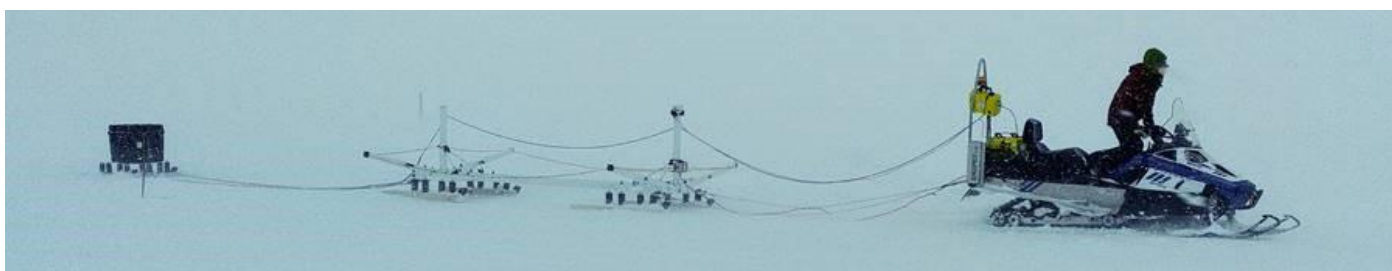
Figure 3. The SnowTEM system. The runners of the sledge have been widened to act as skis and the system is pulled by a snow scooter.
