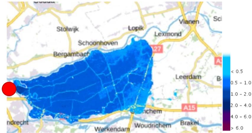
Figure 3.3 Example scenario of flooding by storm surge at sea, dike breach (red dot) at Kinderdijk (source: LIWO)
