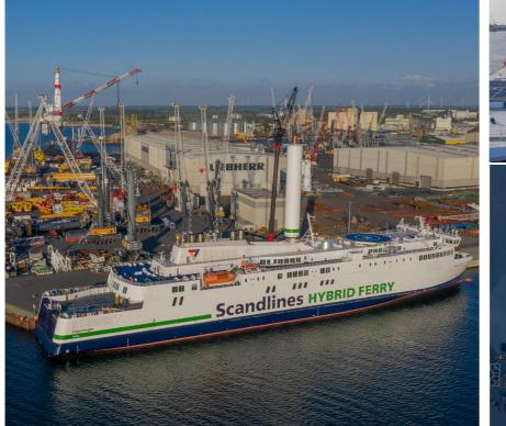
n the 25 May 2020, the Scandlines ferry, MV Copenhagen made port in Rostock to be transformed overnight into a wind-assist hybrid vessel. The installation of the large 30m tall Rotor Sail supplied by the Finnish company Norsepower Oy Ltd took only a few hours meaning that the ferry was ready for operations the next morning, and this installation is expected to reduce emissions by an estimated 4-5 percent.
