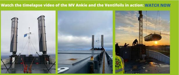
For eConowind BV, located in Groningen, the Netherlands, it is the first commercial installation of their Ventifoil system after a series of seatrials and tests. The windassist system was developed over the past three years supported by
