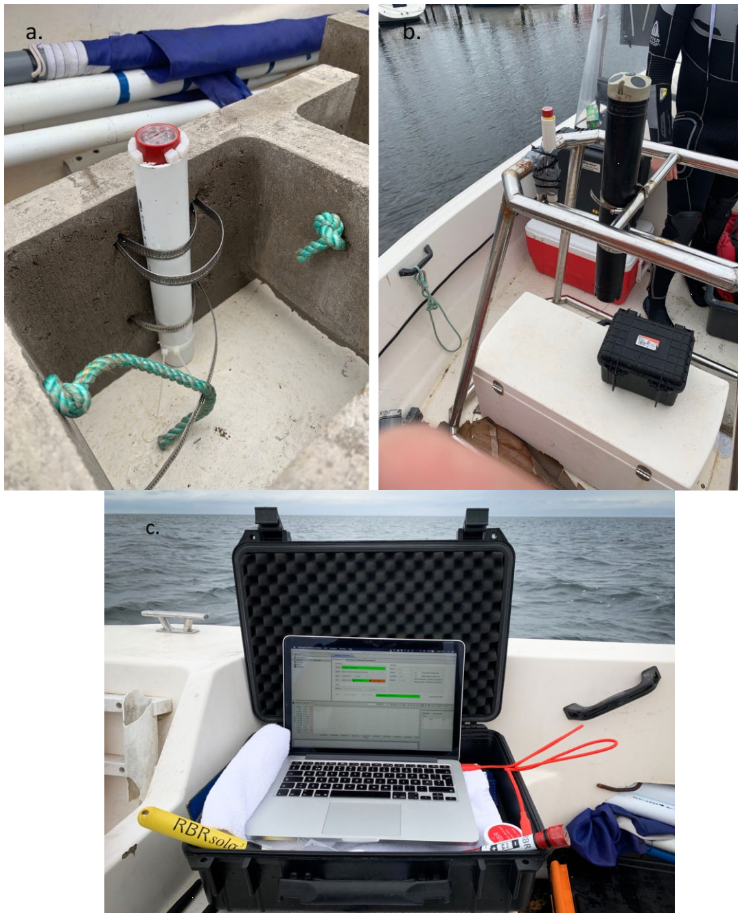
Figure 2. Wave measurements in Lomma Bay, a) deployment of RBR wave pressure gauge attached to concrete block, b) deployment of acoustic Doppler and
