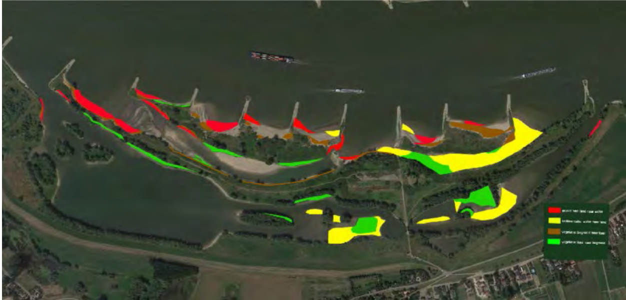
Figure 2.1.3: A result from the detailed study on the Gameraen side channel system. Red indicates erosion, yellow is sedimentation, green is emerged vegetation and brown is disappeared vegetation, always between 2000 and 2019.
