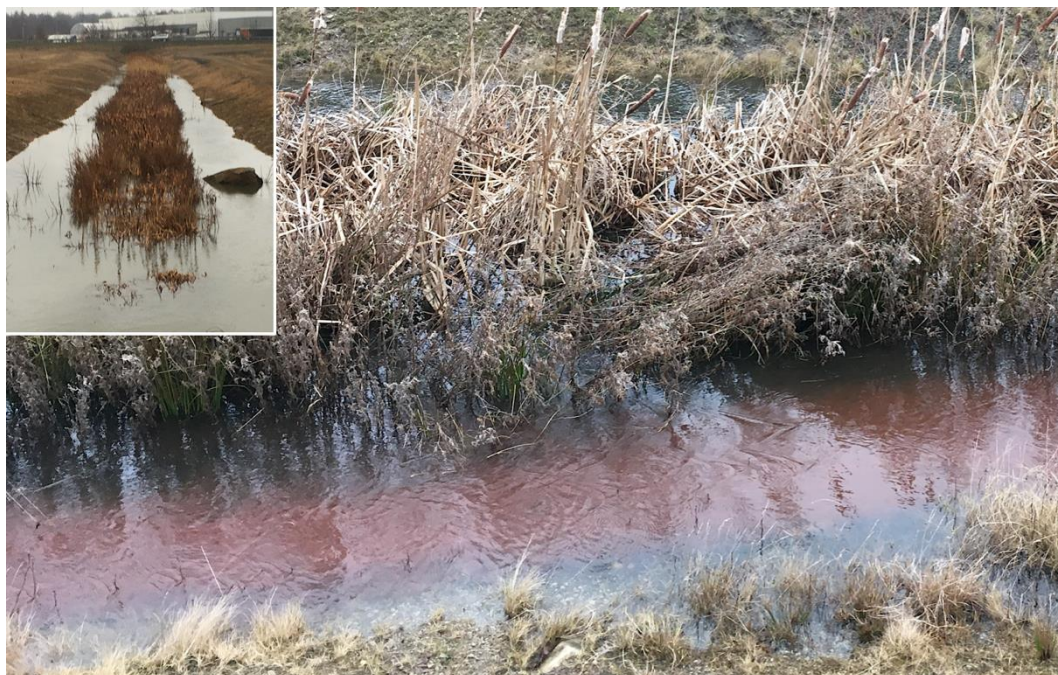
Figure 9 Overbank flow at Site 2 where, as visualised by Rhodamine WT (tracer), the main bulk of the water current is over the bare floodplains due to excessive in-channel vegetation and associated sedimentation. Photos: EA International (February 2019).
