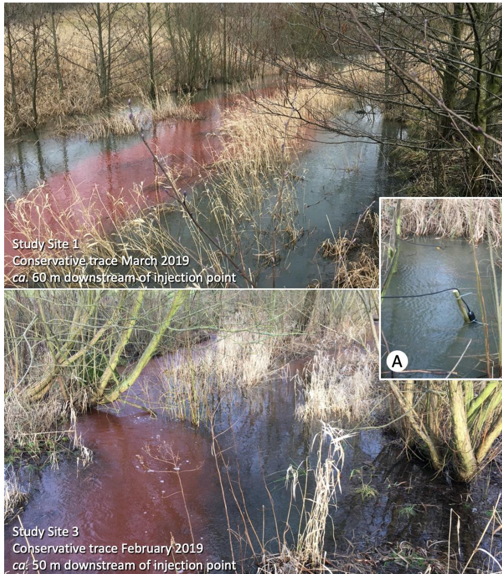
Figure 17 Pictures of overbank flow showing that, although water depth above the floodplain is significant, the majority of the flow (m 3 /s) is in fact confined to the main channel as depicted by the path of the tracer compound some distance downstream of the injection site. (A) Complementary conservative-trace experiment investigating lateral mixing over the floodplain. Photos: EA International (February-March 2019).
