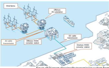
Figure 18 Diagram showing the transmission system from wind farms to landfall point via various cables, substations and converter stations. (Source: ABB)
