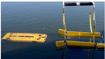
Figure 20 Modus and Osbit. AUV and docking station
