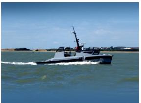
Figure 21 Thales' Halcyon autonomous surface vessel.
