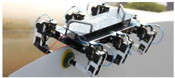
Figure 22 Blade Bug. Wind turbine blade repairs
