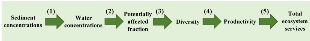
Figure 2. Steps to assess the environmental impact of chemical mixtures in sediments on ecosystem services (ESs) of waterways. Step (1): Convert sediment concentrations into water concentrations. Step (2): Calculate the multi-substance potentially affected fraction msPAF(HC50) of aquatic species based on water concentrations. Step (3): Link msPAF(HC50) to diversity. Step (4): Identify the quantitative diversity-productivity relationship. Step (5): Update the correlation between productivity and the total value of ESs.
