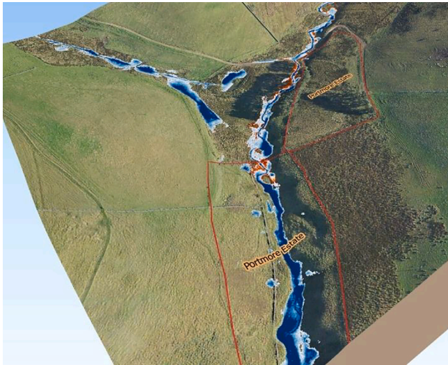
Fig. 10. As more tree-planting increases the friction over 20 years, the orange areas shows flood waters reaching more areas of temporary high flow storage. (For interpretation of the references to colour in this figure legend, the reader is referred to the web version of this article.)
