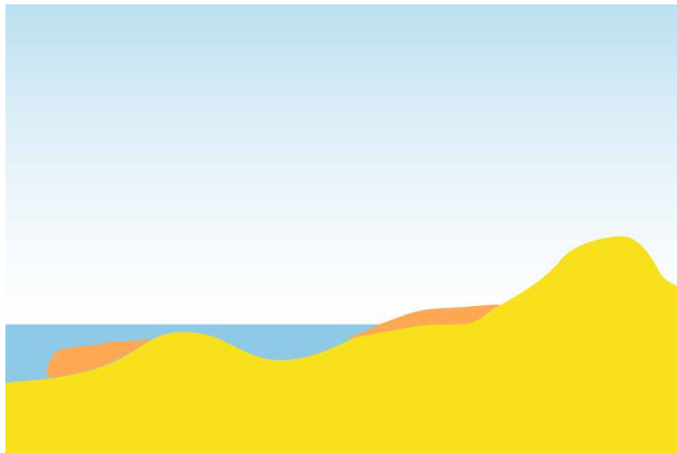
Schematic design of beach and shoreface nourishment, cross-shore
