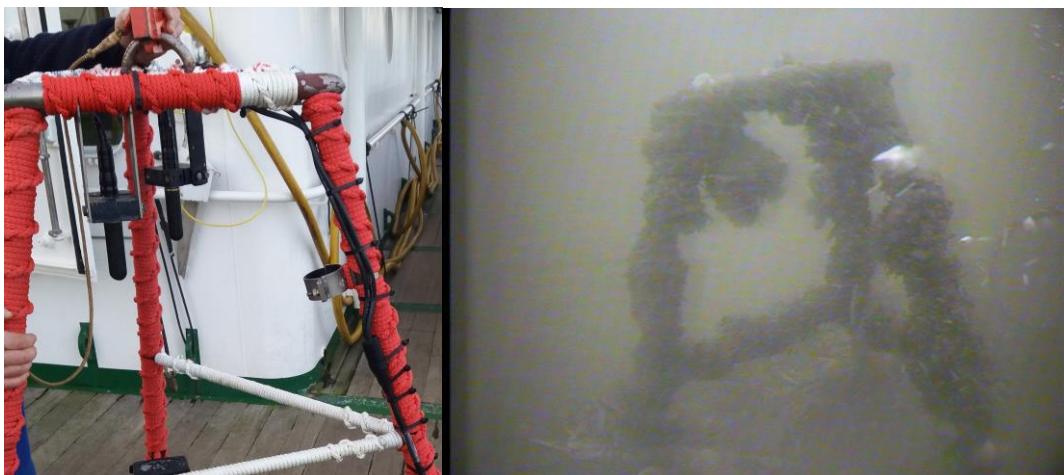
Fig 5: Biofouling on hydrophones in bottom frame after one year operation
