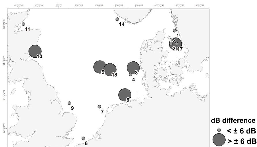
Figure 4.1: dB difference for broadband frequency (20 – 20000 Hz) comparing P50 (median) yearly measurement and model data. Possible reasons for uncertainty at individual stations: 3; proximity to an oil rig, 5; generator at platform, 6; offshore wind farm noise, 10; non AIS fishing vessels, 17; sediment uncertainty in the Kattegat, 18; seismic survey present and proximity to oil rig.
