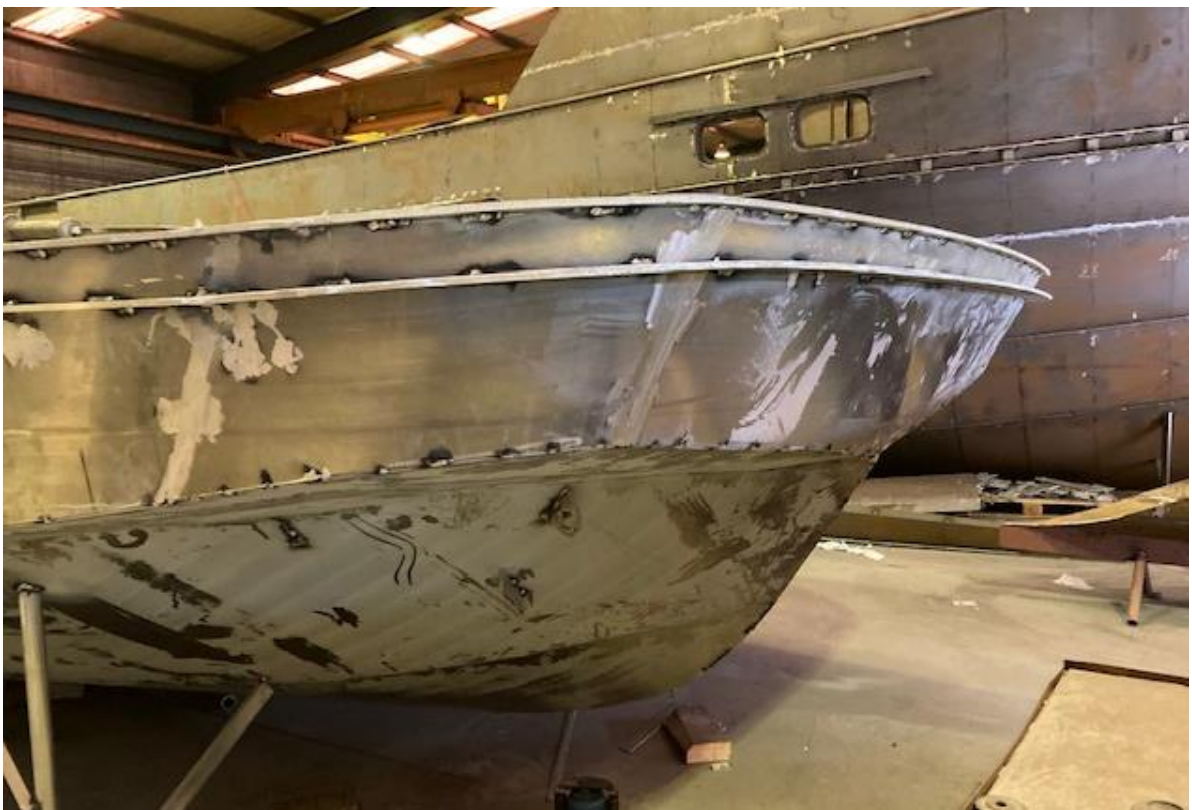
Finishing deck and welding place for rubber protection
