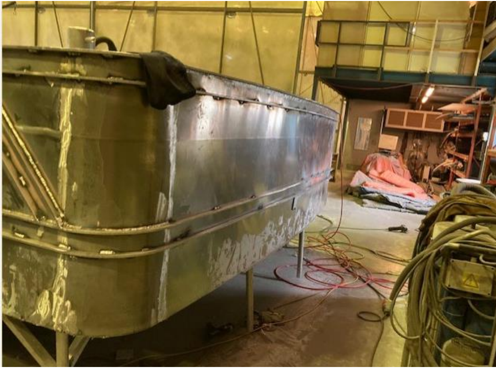
Finishing deck and welding place for rubber protection
