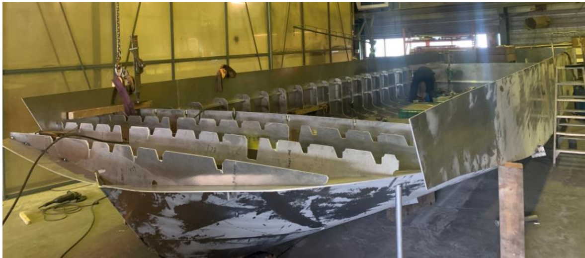
Welding the hold of the hull
