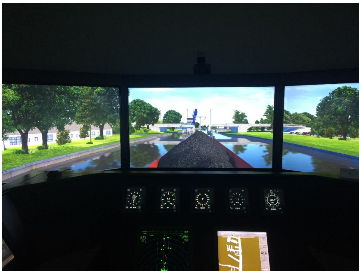
Picture 4: Simulation of a vessel passing a drawbridge on the "Wilde Greuns" waterway in the city of Leeuwarden (IWT simulator MAH for the Interreg NSR project # IWTS 2.0, 2019).
