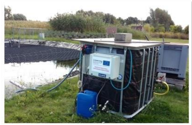
Photo 1: Set-up of Moving Bed Biofilm Reactor (MBBR) at PCS Ornamental Plant Research
