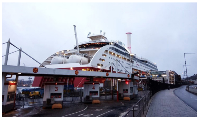
Figure 1: Viking Grace was retrofitted with a rotor sail in 2018
