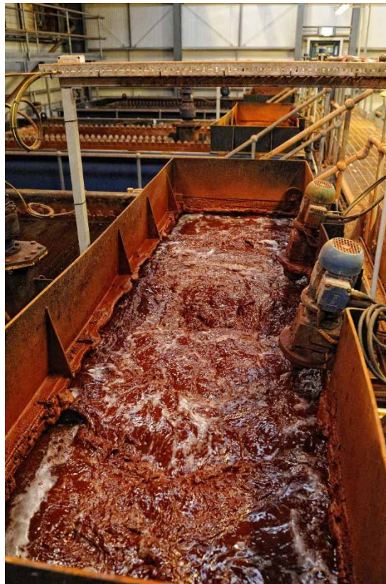
Figure 12 Recharge and cleaning of abandoned mine-water to protect drinking water wells (UK).
