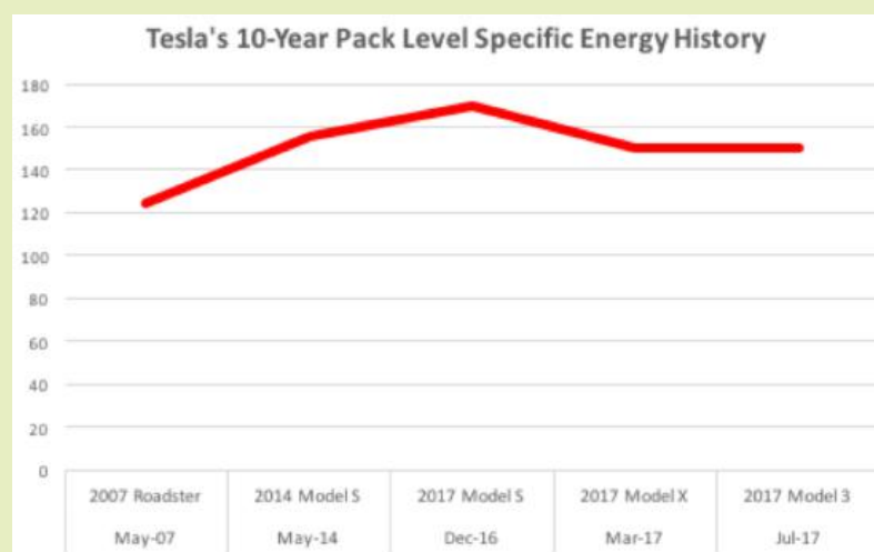
Figure 2. The specific energy density of batteries in different models of Tesla moving forward in time showing that battery improvements are difficult to achieve [5].
