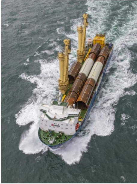
Fig. 24 HLV transporting monopoles, from [58]
