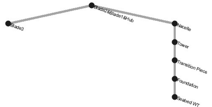
Fig. 9. Wind turbine removal by 6 cut and lift operations by combining two blades and the hub
