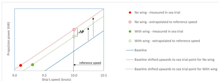
Figure H. Example of how speed trial result is extrapolated to nominal speed using the shape of the Baseline curve.
