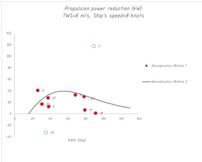
Figure J. Power savings derived with normalization method 1 and 2 at nominal conditions. Reference wind speed 8m/s at 10m above sea.
