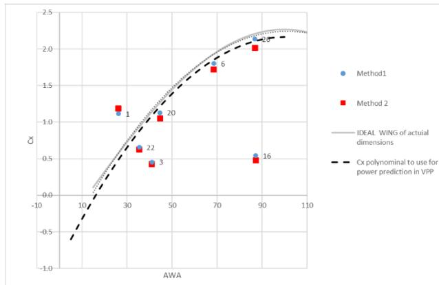
Figure I. Thrust force coefficient derived indirectly from sea trial. Regression found by adapting the  $C_t$  curve of a generic wing forces from SSPA database.
