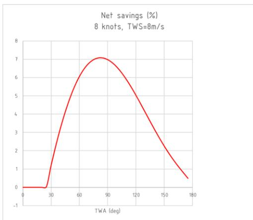
Figure K Power savings derived with normalization method 2 at nominal conditions.
