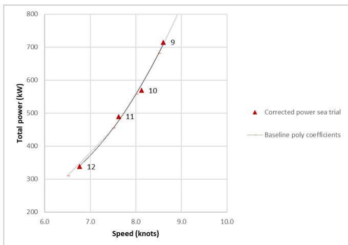
Figure G. Power at sea trial – speed test without wings. Power corrected according to ISO 15016.
