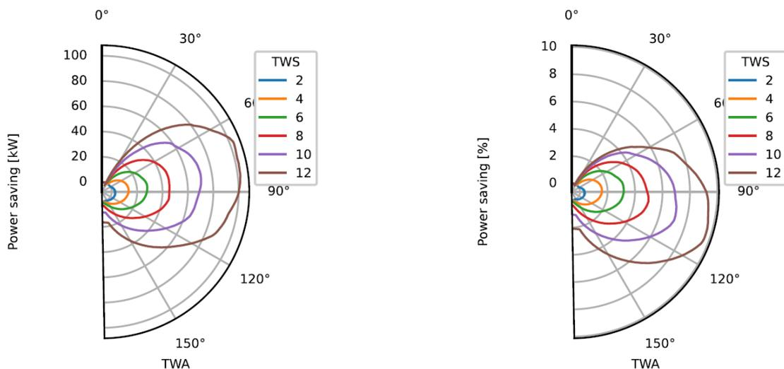
Figure N. Net power saving at various wind speeds.
