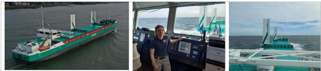
*Figure A. m/v Tharsis (84.45m x 11.4m) with two wings from Econowind. Sea trial on May 26, 2022*
