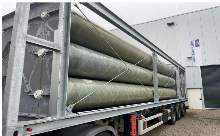
Figure 3 : Containerized Hydrogen Storage for the FPS Maas
