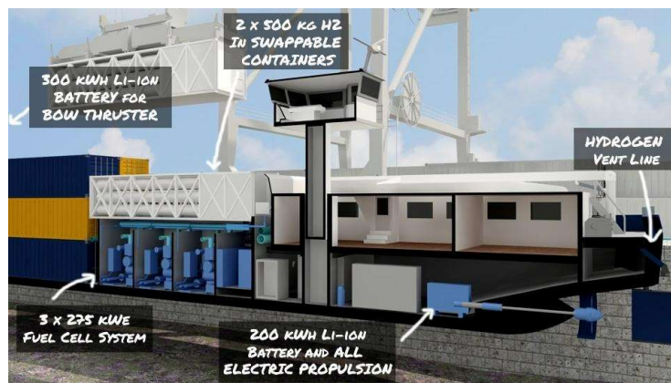
Figure 2 : Side cutaway illustration of H2 Barge 1 Hydrogen system
